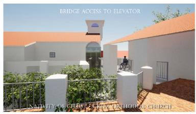
To connect the elevator with the office building, a small bridge will be built from just beneath the overhang. This will allow an easy course of travel from church services to the Fellowship Hall and outdoor patios.
